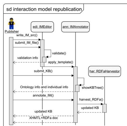
FIGURE 2: Sequence diagram for IM republishing
